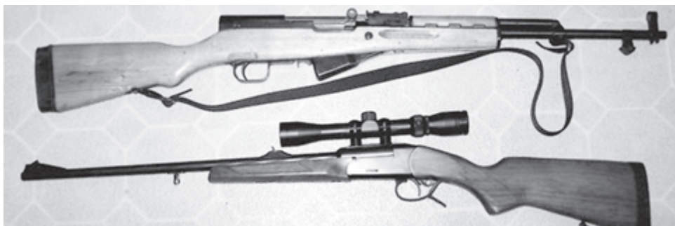
Two rifles available in 7.62x39 are the Norinco SKS semi-auto (top photo) made in China and the Remington Spartan single-shot rifle (bottom) made by Baikal in Russia.
